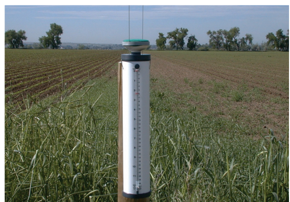
Atmometers provide reference ET at field locations where they are installed.
