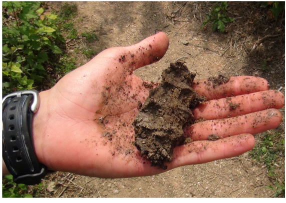
Estimating soil moisture by the hand/feel method.
