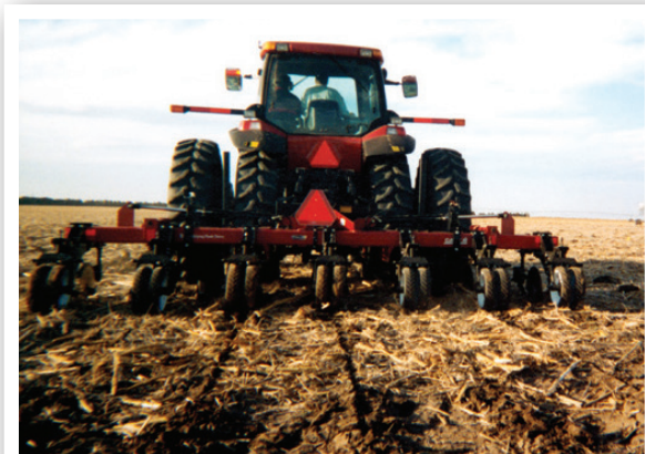
No-till ripper post harvest. Ripping is most effective in dry soils.
